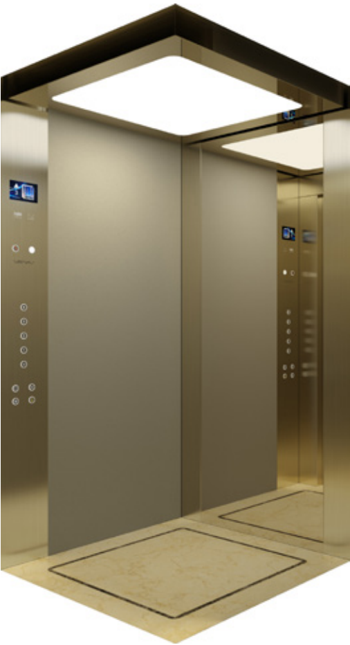
G5306 吊 顶 (G1096)：香槟金镜面不锈钢，亚克力透光板 侧后壁：皮纹化妆钢板 (G4481) 侧前壁：香槟金发纹不锈钢 后边壁：香槟金发纹不锈钢；后中壁：香槟金镜面不锈钢 地 板 (G3369)：印花PVC（金碧米黄+深啡网纹） Ceiling (G1096): Champaign gold mirror stainless steel, Acrylic Side Back-wall: Leather decoration panel (G4481) Side Front-wall: Champaign gold hairline stainless steel Rear Mid-Wall: Champaign gold mirror stainless steel Rear Side-wall: Champaign gold hairline stainless steel Floor (G3369): PVC
